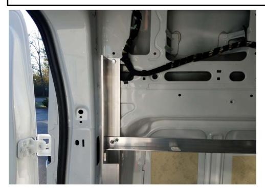
NOTE: For Box Truck installations no hardware is supplied. Every truck is constructed differently and uses different materials. The basic procedure is to use 4 bolts fastening through the wall itself, the top two bolts should be fastened to the "roof sidewall member"
