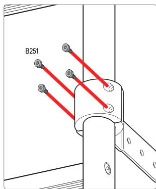
Do not completely tighten bolts so adjustments can be made later on.
