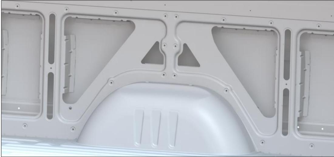
*"Vehicle's bare metal in the wheel well area" This is view from inside the vehicle*
